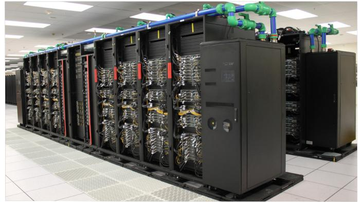
**Magma, with 760 compute and user nodes plus 12 management and file access nodes, is a liquid cooled supercomputer built by Penguin Computing featuring Intel® Xeon® Platinum processors and Intel® Omni-Path Architecture fabric. (Photo courtesy Lawrence Livermore National Laboratory/Meg Epperly)**
