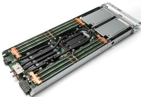
**Innovative cooling technology offers high serviceability and provides very stable liquid cooling across the DIMMs.**
