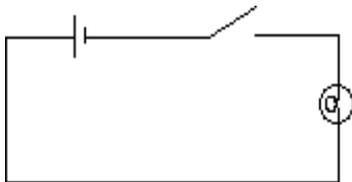
In this circuit, the wire is the conducting path, the battery is the power source, and the bulb provides the electrical load. The action on the circuit is controlled with the switch. When the switch in this circuit is closed, there is a complete electrical path from the battery to the lightbulb and back to the battery. The bulb will light up as the current flows through it. If the switch is open, the circuit pathway is incomplete and the bulb does not light up.
