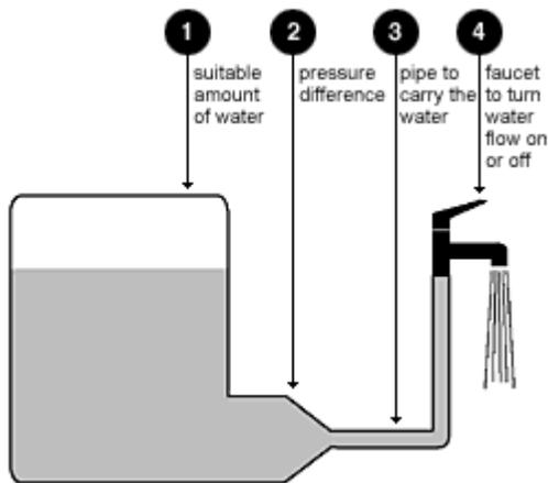
Electrical current in a circuit behaves like water flowing in the water pipes of your house. Getting water to the kitchen sink requires four things: a suitable amount of water, a pipe to carry the water, a pressure difference between the source of the water and the tap, and a tap to turn the flow of water on or off.
