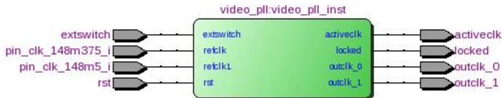
The above PLL has two reference clocks `pin_clk_148m375_i` and `pin_clk_148m5_i` and the PLL switches between these two clocks.
