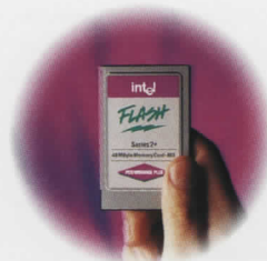
Intel's flash memory card can replace the disk drive in mobile computers, storing the equivalent of 27 high-density floppy disks full of information in a credit-card-sized package.
