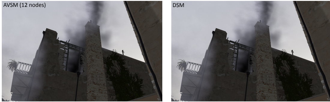
Figure 3: A comparison of smoke added to a scene from a recent game title with AVSM with 12 nodes (left) and deep shadow maps (right). Rendering the complete frame takes approximately 32 ms (30 fps), with AVSM generation and lookups consuming approximately 11 ms of that time. AVSM is 1–2 orders of magnitude faster than a GPU implementation of deep shadow maps and the uncompressed algorithm, yet produce a nearly identical result. Thanks to Valve Corporation for the game scene.
