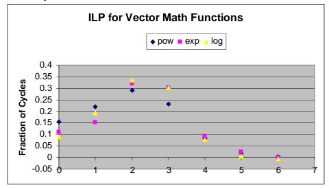
Thus a strategy for optimization would be to minimize the area under a non-normalized form of such a curve by shifting the curve to the right, and achieving greater parallel use of the processors execution units.
